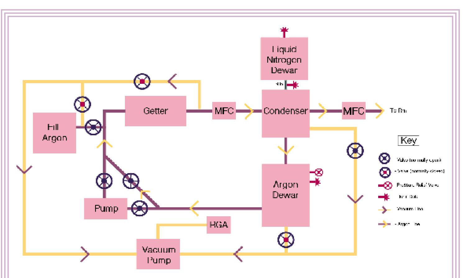
We built a system which uses liquid nitrogen to condense gaseous argon into a liquid and a PID controller (integrated into the Raspberry Pi system) to maintain a stable pressure within the argon dewar at all times.
